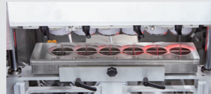
• Air Rinse Station
